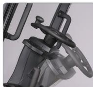
Infinitely adjustable steering column
