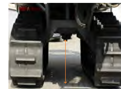
Higher ground clearance (300mm)
