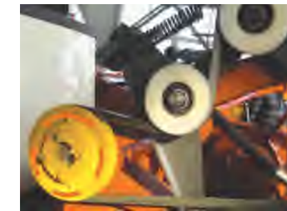
Different RPM of reel (35, 38, 41, 45). Easy to change single belt
