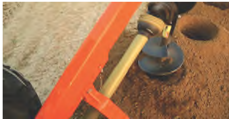
Long lasting, wear resistant auger tip
