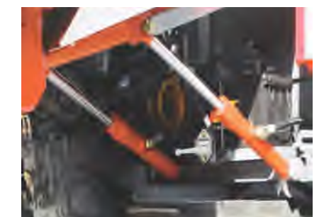
Double oil cylinder header assembly for better stability
