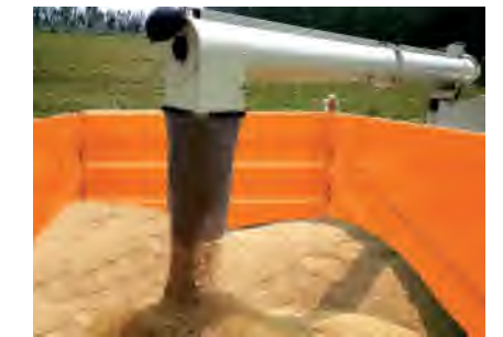
Quick 340° rotating grain discharge auger & hydraulic operated vertical height adjustment
