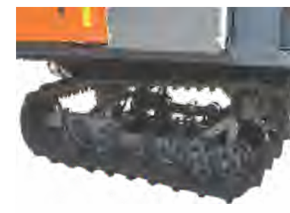
Straw anti-winding design of Rubber Track for good performance in paddy field
