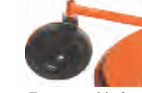
Tyre assembly for depth control
