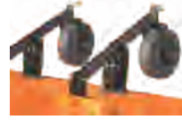
Tyre assembly for depth control
